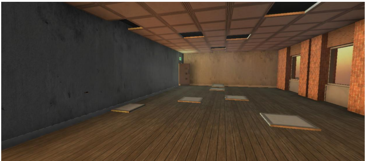
Figure 13: Walls are retextured using higher resolution images. Similarly the floor is retextured, using bump and normal mapping to emphasise the divisions between individual boards. To highlight the earthquake scenario individual ceiling tiles are added and given physical behaviours using the same model applied to the player; as the simulation starts these tiles fall and collide with the floor.
